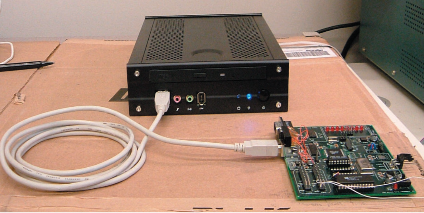
Fig.1 The Problem: PCI control systems required prohibitive cabling and expensive dedicated hardware.
